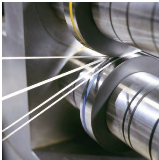
A cut above. Second-generation superconducting wires are slit from wide tapes into thin ribbons.
